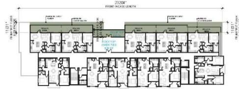
BUILDING A STEP-BACK AREA: 2,095 SF FRONT FACADE LENGTH: 232.25 FT AVERAGE FRONT FACADE STEP BACK: 2,801/232.25 = 11.97 FT
