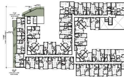
BUILDING C STEP-BACK AREA: 2,073 SF FRONT FACADE LENGTH: 114.75 FT AVERAGE FRONT FACADE STEP BACK: 2,373/114.75 = 18.87 FT
